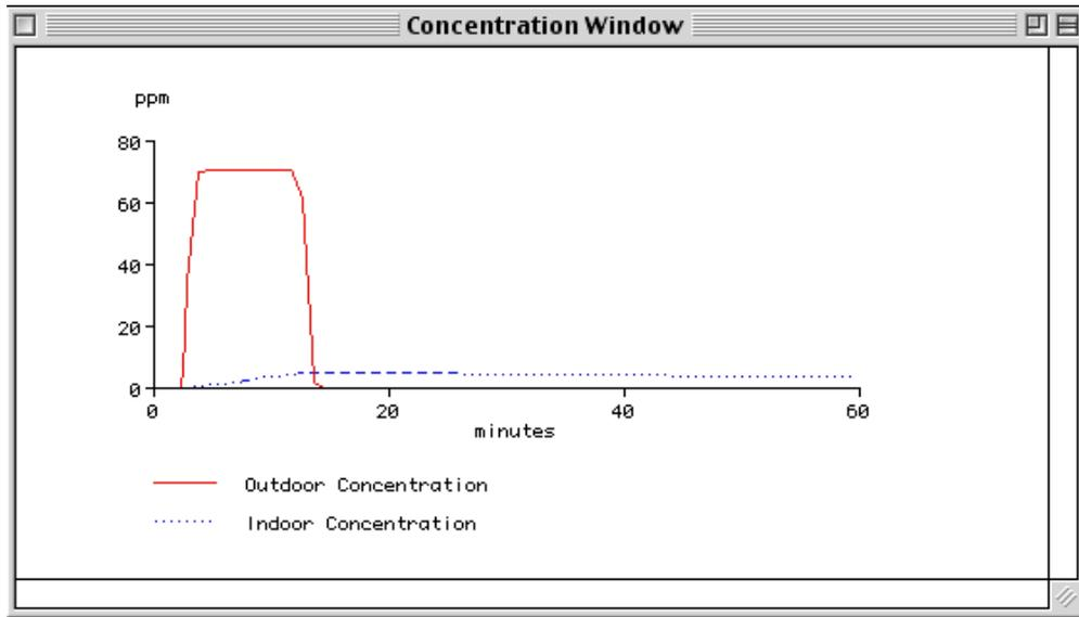
You can see from the graph that the chlorine cloud passes by the office building within the first 15 minutes after the release begins. After that time, the predicted outdoor concentration drops back to zero, while the predicted indoor concentration persists for much longer.
