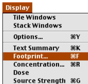
The selected chemical, methane, has TEELs (Temporary Emergency Exposure Limits) as default levels of concern. Click on the **Red Footprint LOC** and choose **User specified**. Put in **5000 ppm** (or 1/10th the Lower Explosive Limit LEL) for the LOC value. Modify the **Orange Footprint** and **Yellow Footprint LOC** values to **(none)**. Click **only for the longest footprint** for **Show confidence lines** and click **OK**.
