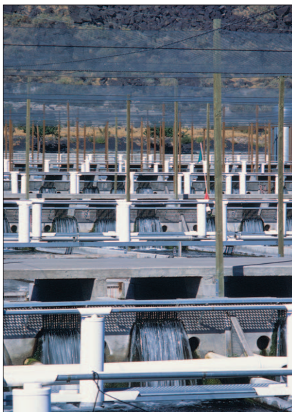
Flow-through raceways are used to raise fish for commercial sale in Idaho. (Photo courtesy of Clear Springs Foods, Inc.)
