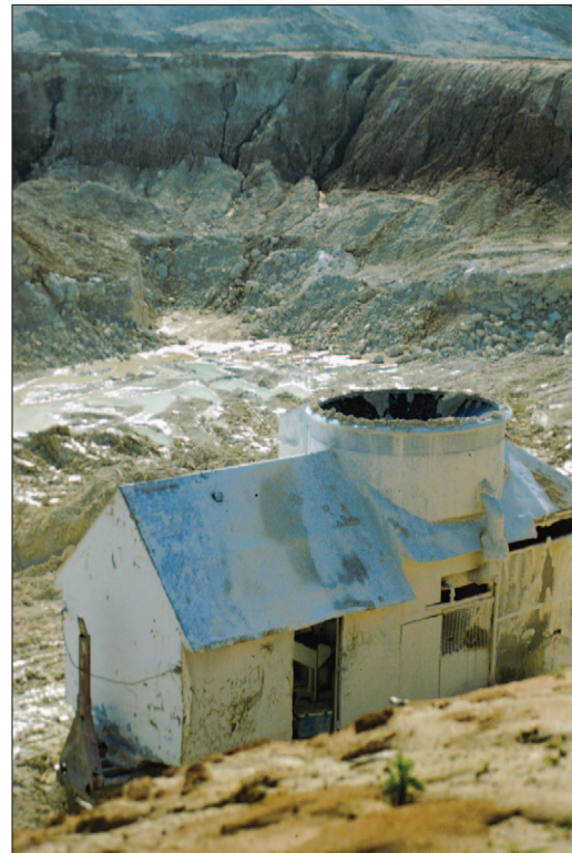
Blunger in kaolin pit, Freeport Kaolin, Gordon, Georgia (Nancy L. Barber, USGS).
