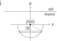
The top lies 1 meter below the surface. Let the origin (0,0) be the top center of the plate. The radius is 1/2, so the lower boundary of the plate is  $y = -\sqrt{1/4 - x^2}$ . The depth of the y-slice is 1 - y.
