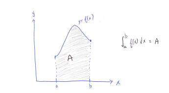
The graph above is for the case when f(x) takes only positive values. If f(x) takes on both positive and negative values then the definite integral will represent the sum of the areas of the rectangles that lie above the x-axis and the NEGATIVES of the areas of the rectangles that lie below the x-axis. This difference of areas is called the net area. Using graphs we have:
